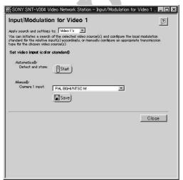
If only the current video source is to be set, select [Video 1's] in the [Apply detection and settings to] drop-down list. Otherwise, if all video sources are to be set together, select [All Videos']. Then select the modulation method for the video input: either by manual setting or automatic detection.
